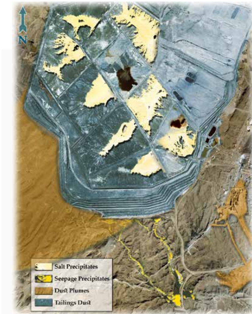
Figure 13: Areas of potential dust generation in the vicinity of the TSF.
